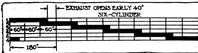
Fig. 16—Chart of overlapping power impulses which is approximately correct for a six
